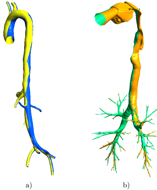
Figure 6. Examples of the multiscale Laplace partitioning method applied to geometries with large geometrical aspect ratio \eta : a) aorta ( \eta = 17 ) and b) human airways ( \eta = 89 ).
