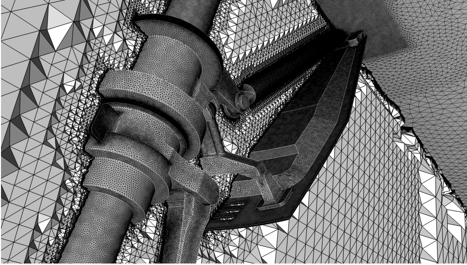
Figure 19. Remeshing of a landing gear. Figure shows part of the 3D mesh boundary layer mesh around the landing gear.
