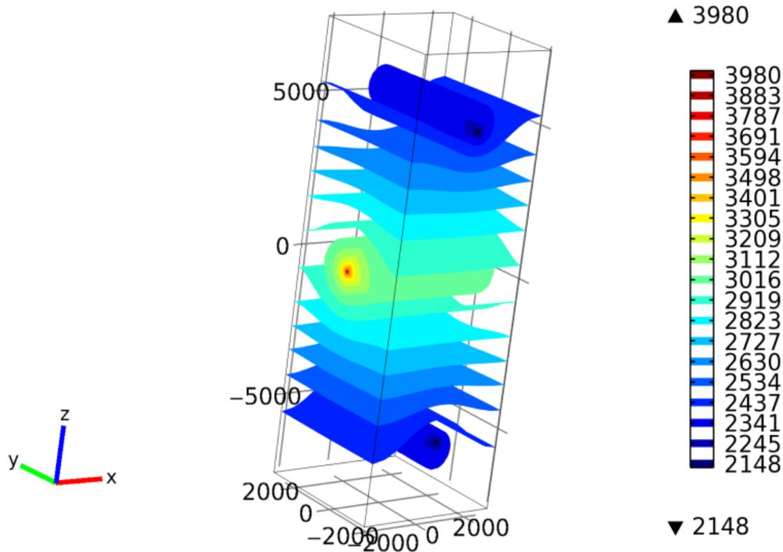
Figure 2.3: Electric equipotentials (V) for a unit cell of the bulk MWPC. The spatial axis scale is in units of  $\mu m$ . The two cathode wires are held at 2100 V and the anode wire is held at 4028 V.
